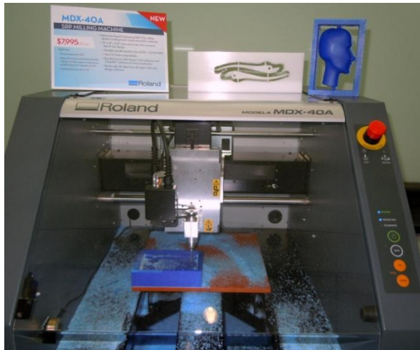
The $8k Roland Milling Machine carves a plastic model from an image captured by the Z-Scanner http://www.youtube.com/watch?v=Yir7T165RcY
